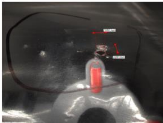
Picture 2: Cut through the film and a few notches in film surface
